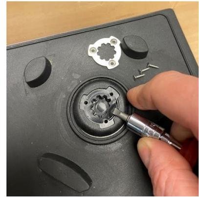
Hold the motor drive (20) in position with multiple slip joint pliers, and unscrew the fixing screw (19) using a TORX wrench (anticlockwise)
