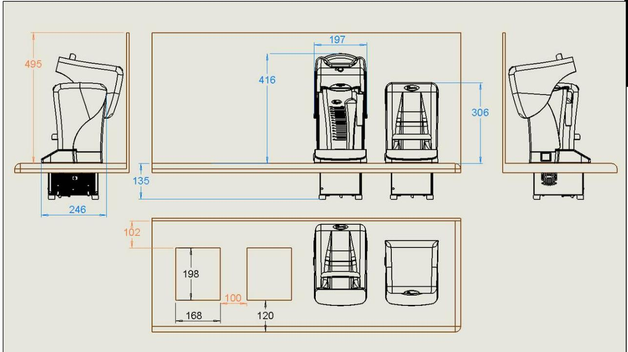
Make sure there is sufficient clearance (behind, above, below) for proper installation and operation of the appliance.
