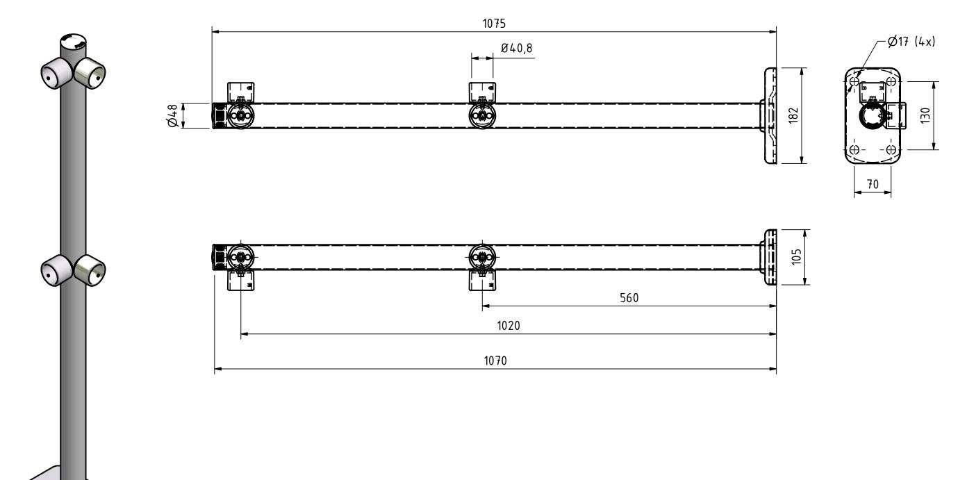
Self drilling screw R6B Twin Fast 10346-00 Upright chrome Ø48 1080 11002-10 2 4 Tube socket concave R24 chrome 10214-10 Title Part number ltem Material Drawer 109mure Where no tolerance is specified: SS-ISO 2768-m Designer Replaces Replaced by Upright, 4 cups, Corner RH Ø48 Date 2009-09-28
