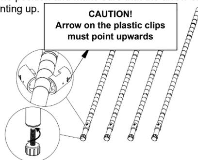
② Please make sure the wire shelf (A) is the correct way up (keep the gap in the collar facing down). Hold the wire shelf on its side and slide the top of the four lower poles through the bottom of each wire shelf as its corner until it snug fits. After four poles have been slide through the shelf collar holes, set the shelf upright.
