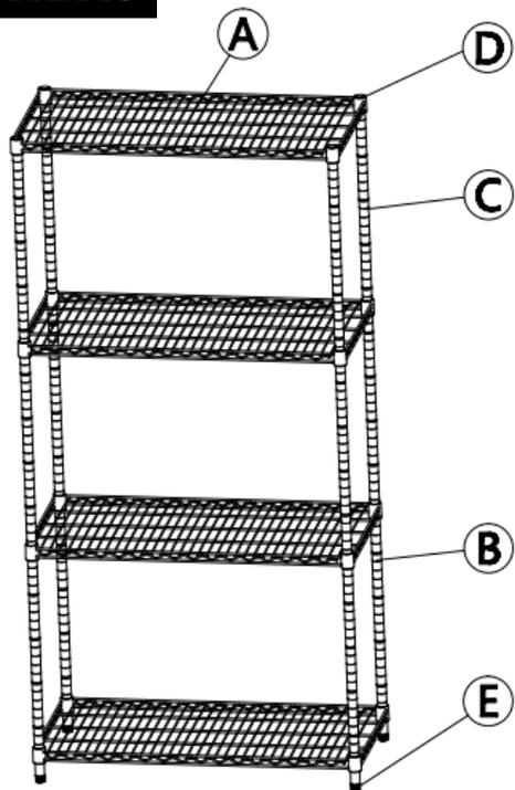
① Screw the levelling feet (E) into the bottom of the four lower poles (B) Snap the plastic clips (D) into the pole grooves of the four lower poles at the same position and make sure that the arrow on the plastic clips is pointing up.
