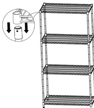
⑥ Once all the shelves have been installed, pushing firmly down on every shelf at the corners with a rubber mallet to ensure the shelf is in place over the plastic clips. Screw the levelling feet in or out to attain proper levelling.
