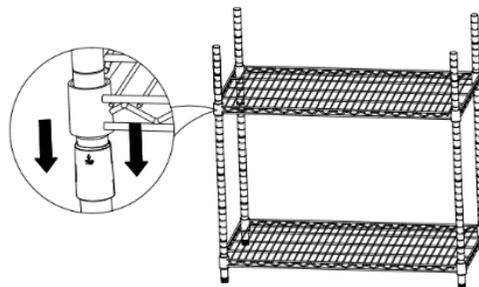
④ Connect the upper poles (C) with the lower poles (B) by screwing the two parts together through the screw connectors which are already present on the upper poles.
