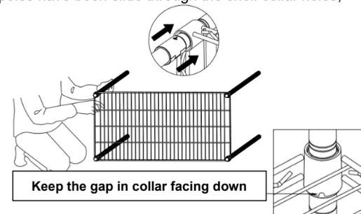
③ Snap the plastic clips into the pole grooves of the lower poles at your desired shelf height/position. Slide down the shelf from top down into the plastic clips.
